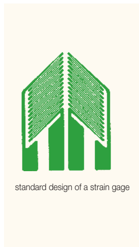
Function principle of the strain gage transducers
